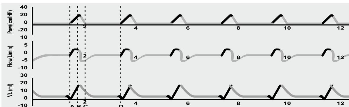
The above picture depicts pressure waveform, flow waveform and volume waveform. A denotes start of inspiration, B–peak inspiration, C- end of inspiration, D-end of expiration
