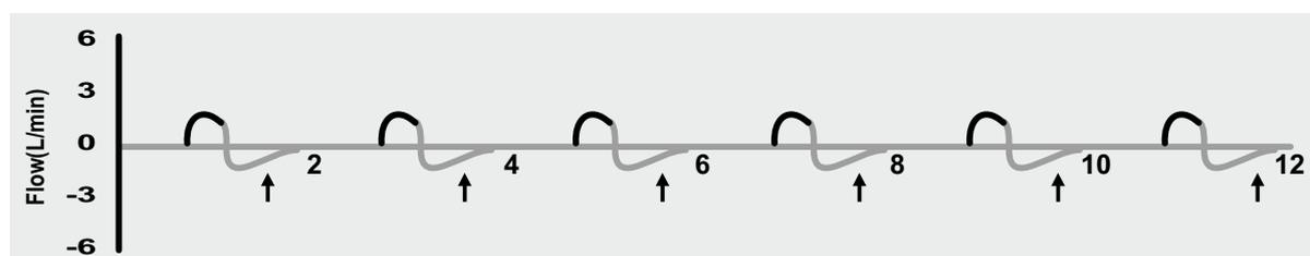
The above picture denotes the decreased slope and increase time for the decelerating slope to return to baseline. Gas trapping
